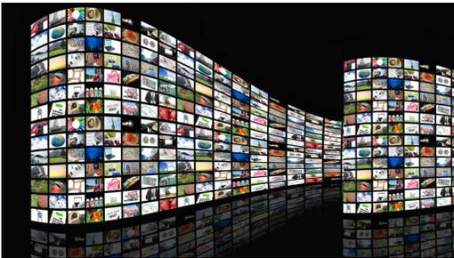
Content can be driven to the screens in a number of ways. Connecting one screen to the next in a daisy-chain fashion can eliminate the need for complex AV equipment, lowering costs and making for easy installation. PC players with multi-head graphics cards allow for native resolution without having to “blow up” content, allowing for much greater resolution. In addition, screens can be controlled individually, with specific content directed at a certain screen or group of screens.
